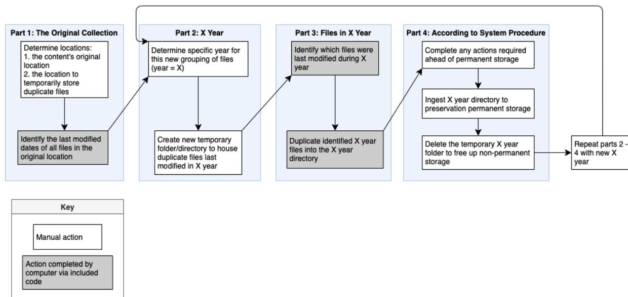
The general workflow consists of four parts, comprising both manual actions (in white) that are completed manually by the person overseeing this process, such as making decisions or indicating folder locations, and actions completed by the computer using code I've written in python. The included appendix provides access to these scripts as well as clear usage instructions for readers' direct use and is summarized and explained in the following subsections.
